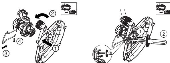
Push the locking knobs and install the auxiliary handle in place.
