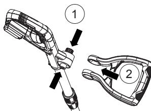
Installing and Removing the Batter Pack Your Battery Pack is UNCHARGED and it must be fully charged once before it is used.
